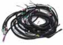
Main wire harness for 11CV BL upto 1952.
