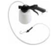
Brakes bleeder device! Working pressure 5-8 bar, max. vacuum 60%, capacity 1L.
