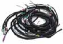
Main wire harness for 11CV BN as from 1952.
