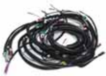
Main wire harness for 11CV BN upto 1952.
