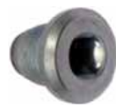
Oil drain screw magnetically, suitably for Citroën 2CV, HY, DS, 11CV (with oil pan out of sheet metal). Interior square. The suitable tool has our number 20221. Or. No. A1321M, thread M16x1,5x20
