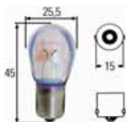
Bulb 21Watt, front indicator, rear brake light, 12 Volt, Ba15s
