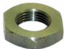
Nut from high-grade steel, for wiper axle outside. Suitably for Citroën 11CV, 15CV. Dimension: M8x5x0,75. Nr.721191
