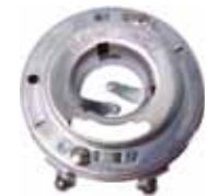
Bulb socket for the headlamp MARCHAL. Suitably for Citroën 11CV and many other French vehicles. Base Ba21d + additional support for a Sofitte for the parking light. Suitable bulbs for the main headlight: 14353 6 V 40/45Watt - color yellow. 14076 6 V 40/45W clearly. For the parking light: Sofitte 14426 6 V.
