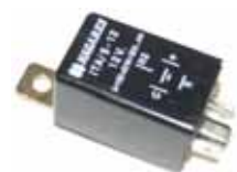
Flashing relay for use a trailer, 12 V. French version! Connection French: Current supply symbol (+). Connection indicator in front + rear = symbol (C). Connection control light dashboard = symbol (R). If a Japanese relay is used: Plus + = symbol X or B. Connection indicator C = symbol L. connection control of R = symbol P. Connection German relay: 31 = frame = must be put. 49 = input voltage = +. 49a = out-put voltage to indicator = R. C = control light = C.C2 = additional control light when using a trailer = 31 equal outlet (earth).
