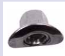
Wheel nut short, galvanizes, suitably for Citroen 2CV, gs, DS. Peugeot 403, 404, 204, 304, 504, 505. Measurement: M12 x 1,25. Fastening torque 2CV: 40-50 nm. Citroën DS + Peugeot 80-100Nm. Lubricate before mounting. Reproduction. Please lubricate before mounting. Replica
