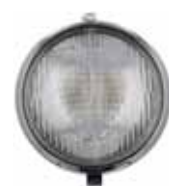
Auxiliary headlight: Fog headlight small, type Marchal 640. Optically like original. Universal fitting. This headlamp was an original related accessory for Citroën 11CV. Diameter: 140mm. The case is chromium-plated and made of metal. Without „E“ test character! Suitable bulb 12 Volt= 14415, 14418, 14417. Bulb 6V = 14178
