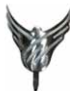
Crank hole cover in grille for 11CV BL, Or.No.: 331137
