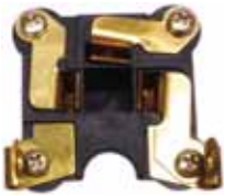
bulb holder headlamp CIBIE 11CV, DS, Peugeot, Renault.
