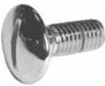
Radiator grill screw (stainless steel) for 11CV/15CV, head diameter: 20mm, M8x25, Citroën No.: 33110, also universal suitable e.g. bumper Peugeot
