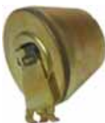
Float from copper, in the carburetor, for Solex carburetor 30/32/34-PICS/PCIS. Diameter above: 37mm, down: 25mm, float height: 27mm. Installed one e.g. in 2CV4+6, Peugeot, Dauphine etc.
