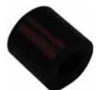
Hydraulic line rubber 6,35mm, LHS (red). 12mm outside diameter. About 10mm long. Only suitably for Citroën DS, with LHS hydraulic system. This heavy rubber is for the connection at the brake system accumulator. Or. No. D392-9020
