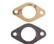
Carburettor base gasket oval, ID19, HY, 11CV. diameter: 34mm, stud center to stud center circa 61mm, also suitable for a lot other vehicles with 34mm Solex carburettor. Or.No.: 481717
