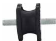
Silent block M8. Diameter: 40mm. Overall height: about 28mm. Thread: M8
