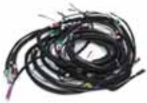
Main wire harness for 15CV BN upto 1952.
