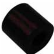
Hydraulic line rubber 6,35mm, LHS (red), 12mm outside diameter. About 10mm long. Only suitably for Citroën DS, with LHS hydraulic system. This heavy rubber is for the connection at the brake system accumulator. Or. No. D392-9020
