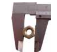
Nut M7, galvanised, 12mm wrench size!
