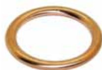
Sealing ring gearbox, for Citroën 11CV/15CV. Suitably for the transmission oil inlet screw + drain plug. 24x32x2,5mm
