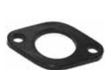
Carburettor base gasket flange Bakelit, thickness: 5mm, inside: 33mm, outside: 77mm, width: 50mm, below Solex carburettor, for 11CV e.g., Or.No.: 481481
