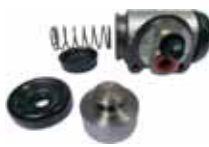
Wheel brake cylinder in front. 1.25 inch (31,75mm) piston. Suitably for Citroën 11CV, of year of construction 1937 to 1957. Mounting board bore: 36,0mm. Brake line connector: 11.0 mm. Length over everything: 68,0mm. Or. No. 621299
