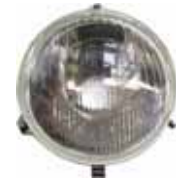
P 403/404/DS, H4 head light unit Peugeot 404, 403 DS >67/11CV, 180mm, version MARCHAL 3 x securement, 1x clip, mounting for H4 glow means, thereby substantially better light! Reproduction without test characters!
