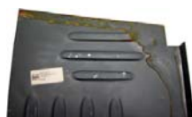
Floor pan bottom surface, in front on the left, Renault R16.
