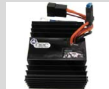
Potential transformer (electronically controlled), from 6 V to 12 V (for a radio. Performance delivery max. 75 Watt). You can use a 12 V radio in a 6 V car!
