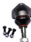
R8/R10/Alpine 110, ball and socket joint above, for Renault R8, R10, Alpine A110. Pin height to area for screwing: 77mm. Thread height: 20mm. Thread measurement: M12 x 1,25. Or. No. 0996006600
