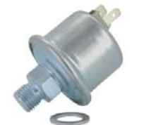
Oil pressure sensor. Measuring range 0 to 6 bar + fixed response pressure 0,60. Thread M14 x 1,5. Suitable for Renault R5, all engines (also Alpine).
