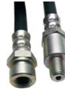
brake hose front R16 65&gt;76 / R12/R15 length 350mm, connection 1 side 3/8-24h inside other side 3/8-24h outside
