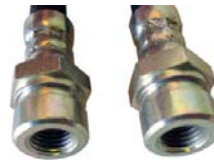
Brake hose rear Renault R16, 220mm length. Reciprocally female itthreads!
