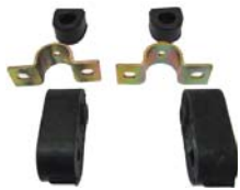
R4, Anti roll bar repair set R4 with 10mm anti roll bar. Contents: 2x clip, 2x rubber bush for clip, 2x hanging up rubber outside, Metal sleeve length = 32 mm. Note: The rubber bush for fixture anti roll bar at the body has always about 15-16mm diameter
