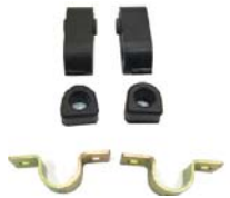
anti-roll bar repair set R4 with 12mm anti-roll bar includes: 2x clip, 2x rubber bush for clip, 2x suspension rubber outside (Metaöl sleeve = 32mm). Note: The rubber bush for fixture Stabi at the body has always about 15-16mm diameter
