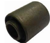
R16/R12, silent beech for the securement of the gear lever. Suitable for Renault R12 + R16. Inside diameter 10mm, outside diameter 22mm, length 25mm, length over all 30mm.
