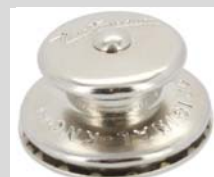
Tenax, snap fastener, upper part, on textile. Very simple and clever system, german invention from 1928. It works like a trailer coupling. The upper part catches a small ball and the system is locked. To open just pull up the upper part. No more brok
