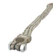
Earth cable (battery ground strap), with battery pole clamp and eye ring. Length: 200mm. Cable diameter: 22mm 2 . Made one in the European Union. Universal fitting.
