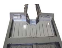
floor panel inner side front, in front of cross bar, Renault R4, with swages replacement for defective panel (sheet metal)
