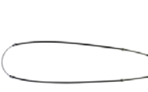
Hand brake cable Renault Dauphine R1090 to year of construction 1963. Dauphine Gordini R1091 to year of construction 1963. Floride R1092 to year of construction 1963. For drum brake. Length totally: 1960mm. Casing length: 2 x 700mm. Or. No. 8544992
