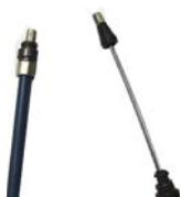
clutch cable Renault 4 TL Cargo >06/66 825/675 mm
