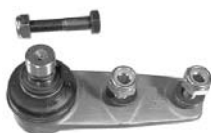
R5 turbo largely, carrying joint front axle, down, on the left of or ion the right fitting. Cone 16mm. R5 turbo 2, with 160 HP.
