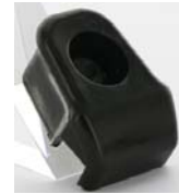
R4/Estafette, stop knob for the sliding window. Suitable for Renault R4 + Estafette. Color: black! Note: It is only the synthetic button, without fixing bolt.
