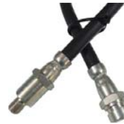
brake hose Renault R4, 5 front 76&gt; for brake discs, length 433mm. connection outer + Inner 3/8 24UNF
