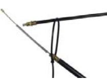
handbrake cable Renault 16 rear left side >74 1170/575
