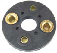
flexible disc steering column R4, 5, 8,16, 18, Dauphine, diameter outer 76mm, inner 24mm
