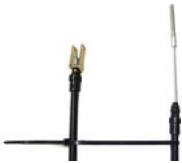
clutch cable Renault 16 69> 560/380 mm
