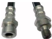
Estafette, brake hose rear Renault Estafette to 10/1967. Connections: 1x 3/8 24UNF inside, 1x 3/8 of 24 male threads. 200mm length, Lockhead Nr.535594
