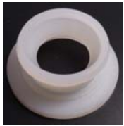
bushing gear shift Renault R4 material plastic (rigid plastic)
