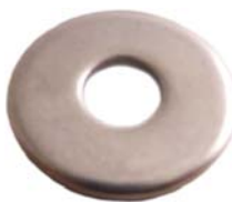
M7, washer largely, from high-grade steel, 7,5x21,5mm, 2mm heavily.
