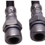
R4/R6, brake hose rear. Suitable for Renault R3, R4, R6. Installed starting from year of construction 1960, 260 - 270mm long. Thread both sides 3/8x24.
