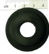
bushing gear shift Renault R4 material rubber
