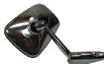
Mirror on the left, chromium-plates. Suitable for Peugeot 204, 404, 504. Renault R4 to year of construction 1985. R5, R8, R10, R16 etc. Hole measurement: 65,5mm. Dimension mirror glass: 163 x 111mm.
