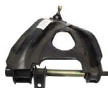
Lateral arm right below for Renault R5 from 1969 to 05/1979
