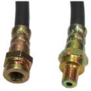
brake hose front Dauphine length 272mm, connection 1 side 3/8-24h inside inside other side 3/8-24h outside
