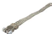
Earth cable (battery ground strap), with battery pole clamp and eye ring. Length: 250mm. Cable diameter: 22mm 2 . Made one in the European Union. Universal fitting.
