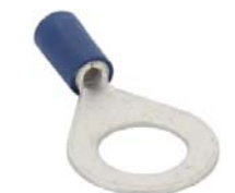
Eye ring blue, 10mm attaching lug. Blue = cable diameter: 2,3 to 5,0mm.
