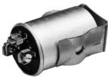
Flashing relay, manufacturer Bosch, round design, for 6 V, performance 2 x 18Watt! Connections: C+49+49a
