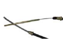
handbrake cable Renault 16 rear right side >70 960/600mm
