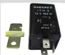
Flashing relay, 12 V, 3 plug connections. 2x 21 Watt power output. Suitable for Citroën 2CV, DS, HY, Renault R4, Peugeot 203, 403, 404 etc. Connection French: Current supply symbol (+). Connection indicator in front + rear = symbol (C). Connection c
