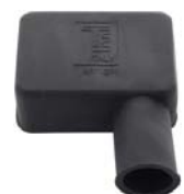
Battery pole protecting cap from rubber. Color: black. Length: 52mm. Wide one: 35mm. Long side left - cable inlet down.
