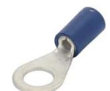
Eye ring blue, 6mm attaching lug. Blue = cable diameter: 2,3 to 5,0mm.
