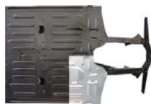
Floor plate front on the left Renault R4
