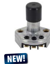
Foot switch for high beam. These switches were often mounted in the floorwell, in order to switch by foot the high beam on. The switch has 3 connecting terminals, with the terminal markings 56a, 56, 56b.
