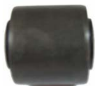
bushing front axle R4, R6, inner dimensions 12 x 27, outside 26 x 23mm. For upper wishbone
