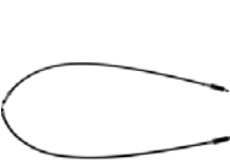
Hand brake cable Renault Dauphine, Floride R1094 + R1095. R8 R1132 + Floride R1131 to Ident. No. 372240. Caravelle to Ident. No. 205187. For drum brake. Length totally: 1900mm. Casing length: 830 + 810mm. Or. No. 8551733
